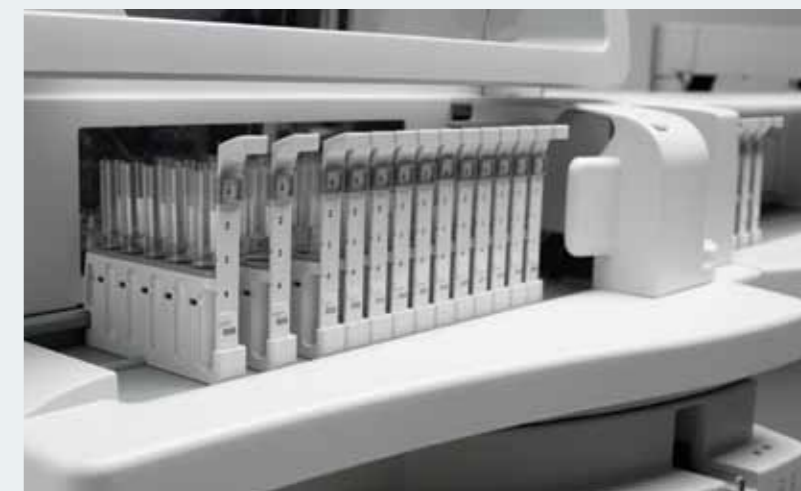
Sample rack holds any size tube
